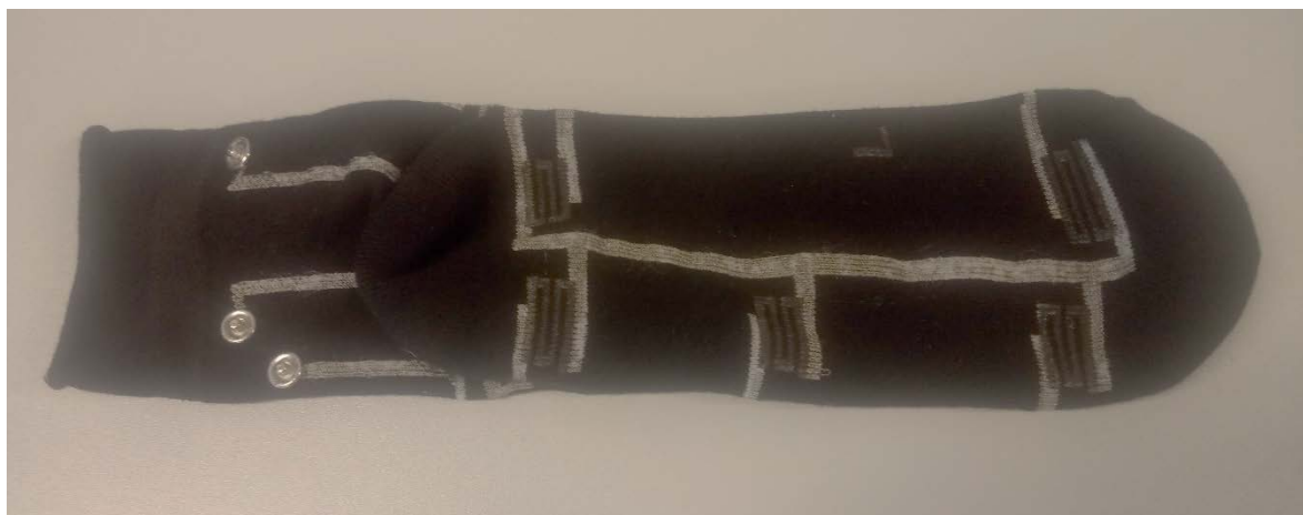
Figure 1 Smart Socks system with 5 textile sensors
