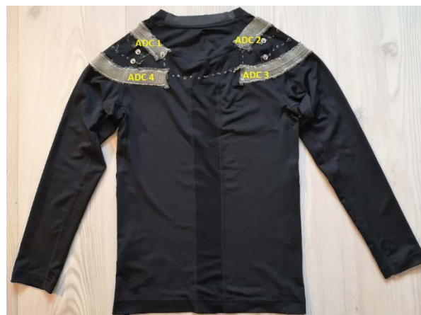
Figure 1 DAid Smart shirt with named sensors
