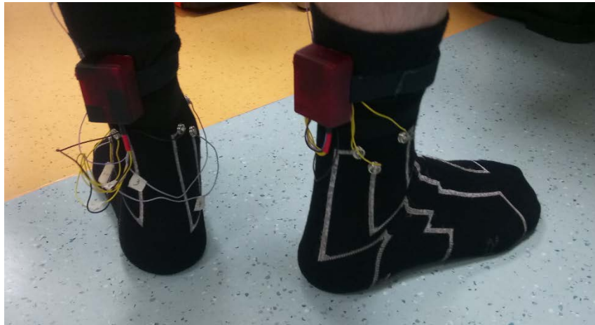
Figure 2 Smart Socks system with the data acquisition box
