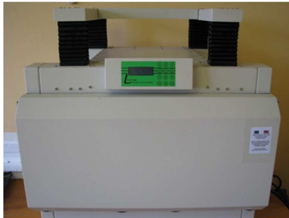
Fig. 1. Heat flow meter instrument 'Laser Comp FOX 600' used in the test of thermal conductivity
