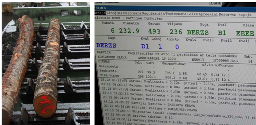
Fig. 7. The example of measuring process and measurement results of identified veneer log N° 24 using 3D scanner system Elmes 3600, where: actual length (cm) 493; nominal length (cm) 480; top diam.u.b.(mm) 232.9; actual volume u.b.(m 3 ) 0.236; nominal volume u.b.(m 3 ) 0.230
