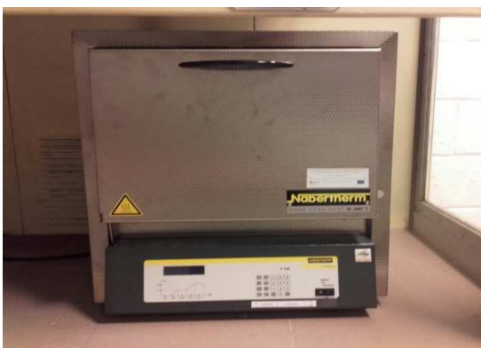
Fig. 2. The furnace used to determine the ash content
