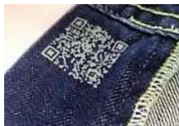
Fig. 13. 2D matrix code directly on the article [44].
