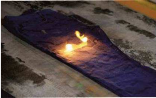
Fig. 8. Laser bleaching on Denim Jeans [21].
