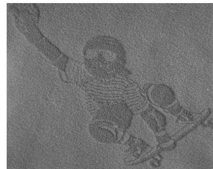
Fig. 10. Laser treating by evaporation (ablation) on polar fabric.
