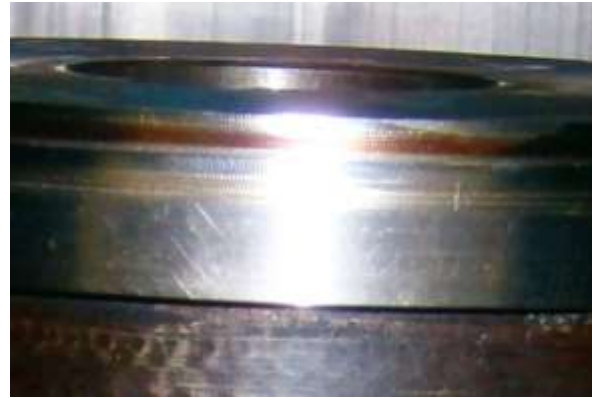
Fig. 7 Marks on the treated surface related to tool wear
