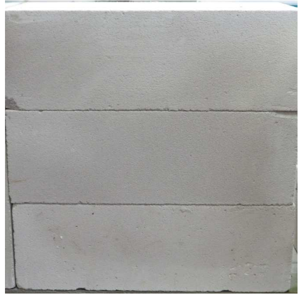
Fig. 1. One of the three aerated concrete sample walls constructed of three blocks.
