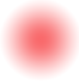
Fig. 2. Normal (Gaussian) distribution of energy within cross-section perpendicular to direction of laser pulse propagation
