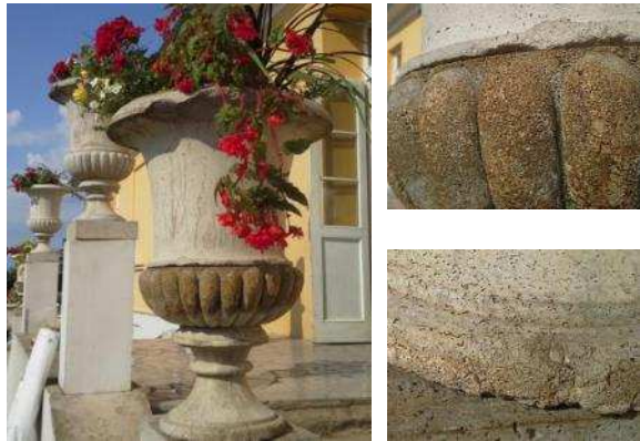
Fig. 1. Vase made from commercially available dry mix after 3 years of exploitation. Typical defects: air voids, cavities and surface erosion after freeze-thaw cycles. (Production – 2011, inspection – 2015).
