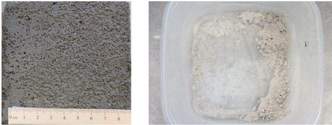
Fig. 5. FC (IP) after 14 cycles of freezing-thawing
