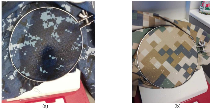
Fig. 1. Surface soaking of the fabric sample (a) and the supplied fabric (b)
