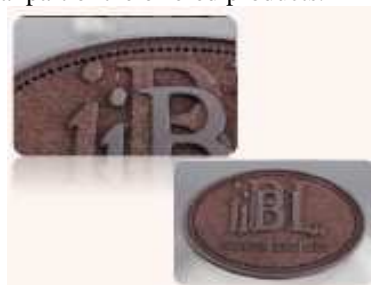
Fig. 14. Laser marking of logo on a leather
