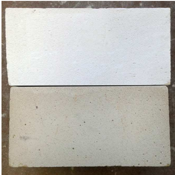
Fig. 2. Aerated concrete sample blocks: above dry and below surface wetted 441 ml during 23 min.
