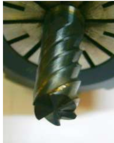
Fig. 8 Wear the instrument after completion of the study
