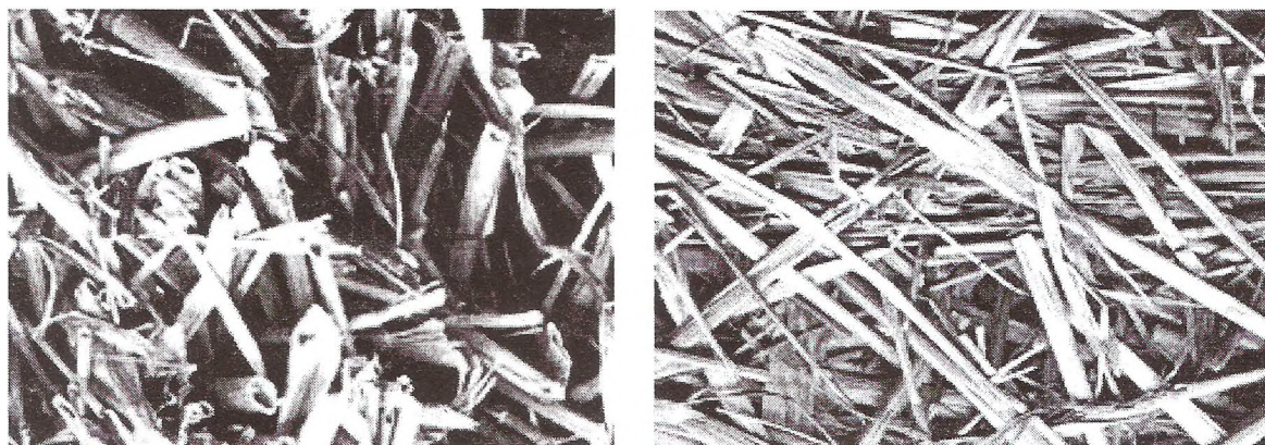
a) b) Fig.1. Orientation of stalks in a straw bale
