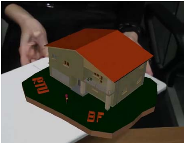
Fig. 3. Three-dimensional virtual model of building in Augmented Reality environment.
