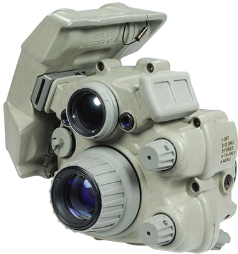
Fig. 4. Enhanced night vision goggle (ENVG) AN/PSQ-20B (last version) [12].
