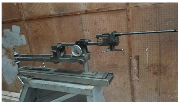
Fig. 2 A stand with a ballistic barrel mounted on it and secured to a foundation.
