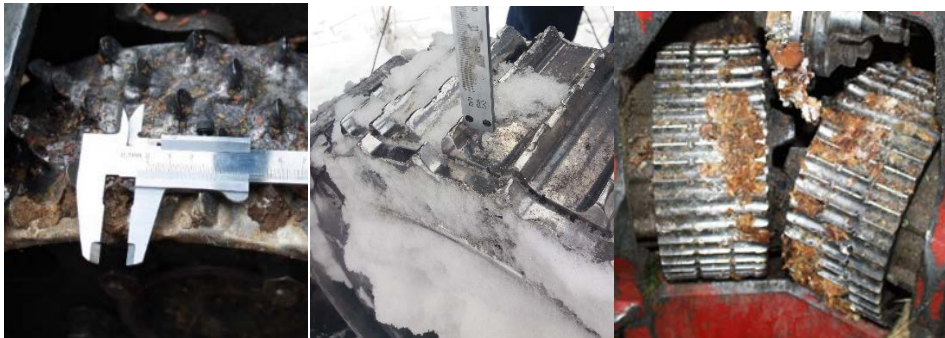
Fig.3. The lenght measurement of the feed roller spikes and evaluation the visual quality
