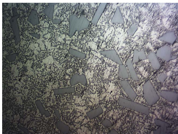
Fig. 6. Structure of the AlSi25 alloy, modified by 0.04% P and 0.05% Sr x200
