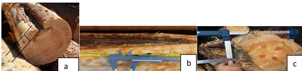
Fig.3. The depth (h) limit of side draught (a) according to the roundwood assortment’s quality requirements: 1cm for wood poles (b); 2cm for sawlogs (c)
