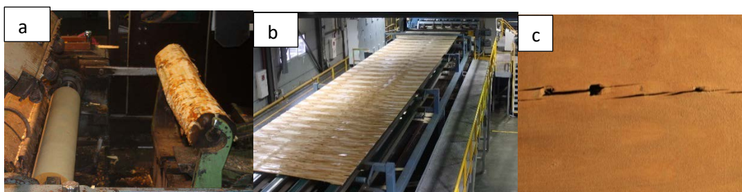
Fig.1. Cut veneer manufacturing process (a;b) and rejected veneer (c) caused by feed roller penetration in timber
