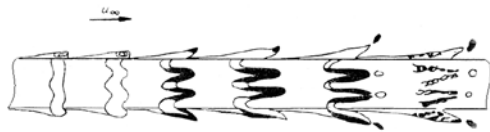
Fig. 1. Visualization of the process of emergence and decay of coherent vortex structures on a body of revolution. Figure from [4]. Quoted from [5]
