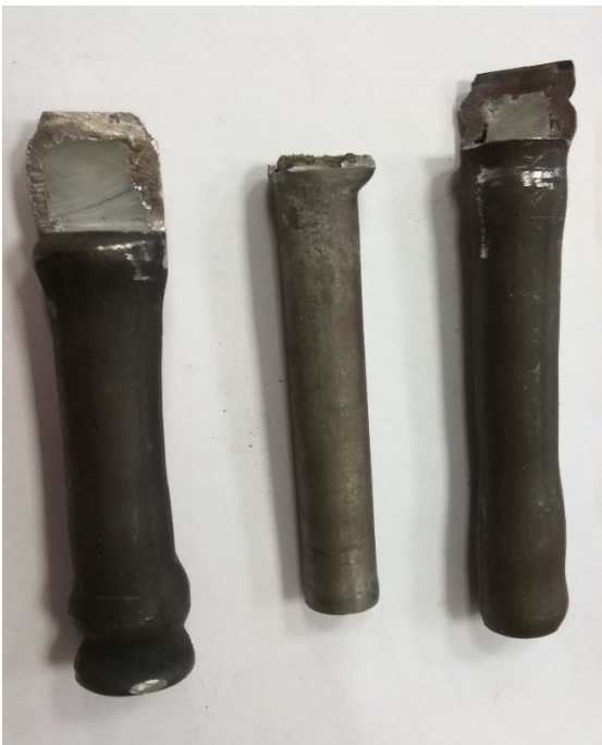
Fig. 2. Specimens made of polyurethane in a metal tube made of steel 10 after dynamic impact in the SDP mode.
