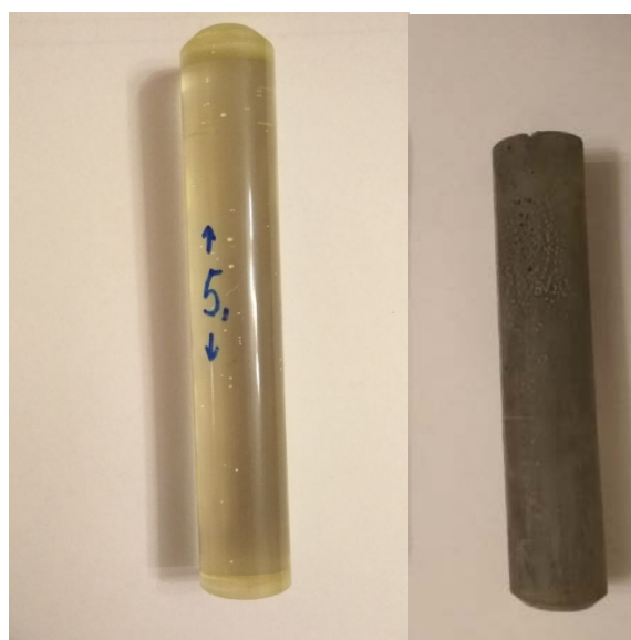
Fig 1. Experimental samples of polyurethane material before and after dynamic processing
