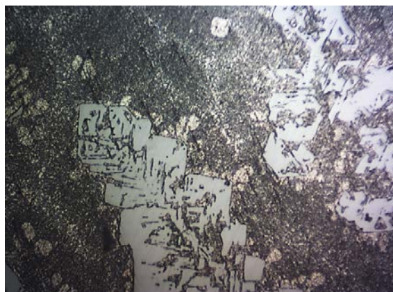
Fig. 5. Structure of the AlSi25 alloy, modified by 0.04% P and 0.2% Ti x200
