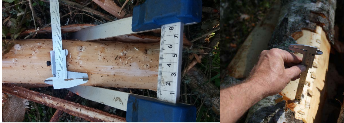
Fig. 4. The measurement of feed roller damage depth in timber
