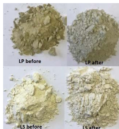
Fig. 1. Dolomite material before and after grinding.
