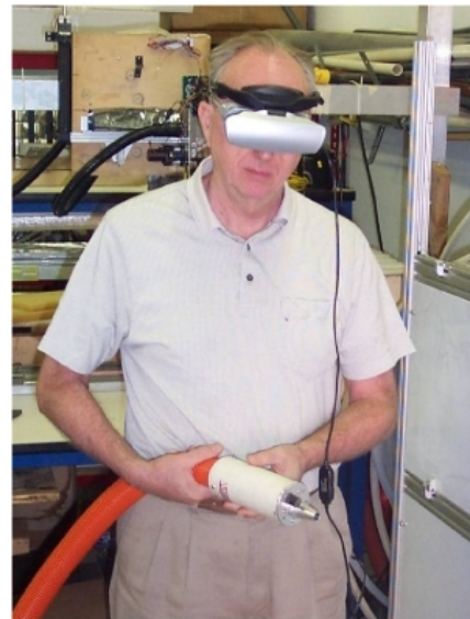
Fig. 6. Heads-up display for confined space access
