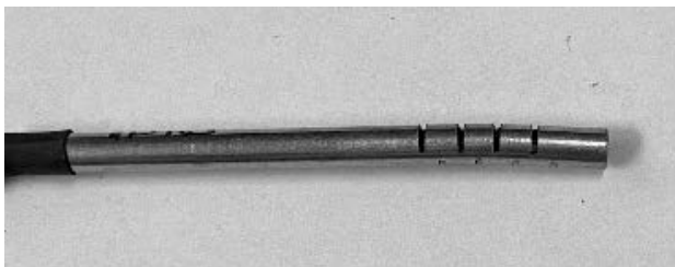
Fig. 3. Semiconductor thermometer based on DS18B20 chip.
