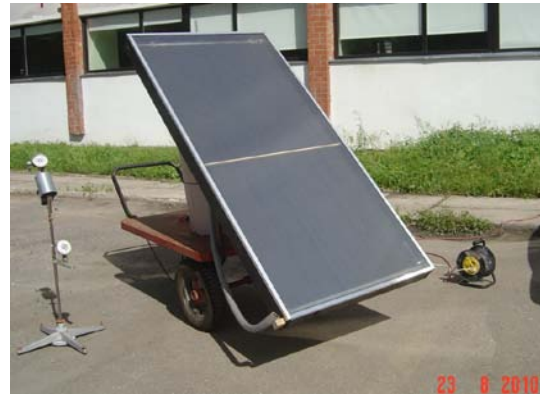
Fig.5. Mobile stand for solar collectors' experimental investigation (look from the outside)
