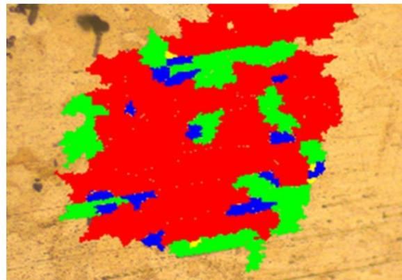
Fig. 4. Software grain measurement after mode №1 after stamping
