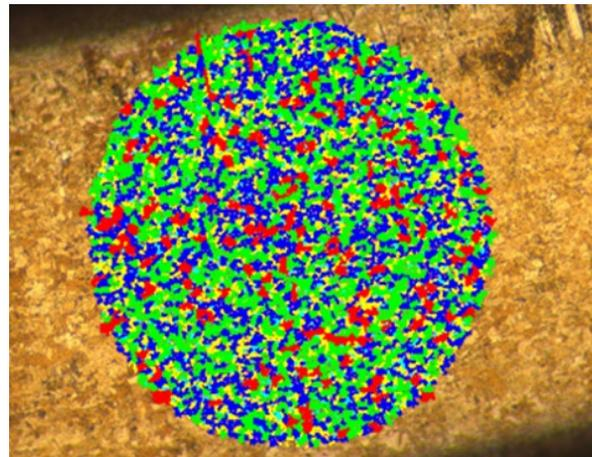
Fig. 1. Software grain measurement after mode №1 after spinning
