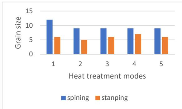
Fig. 5. Results of grain size determination after annealing
