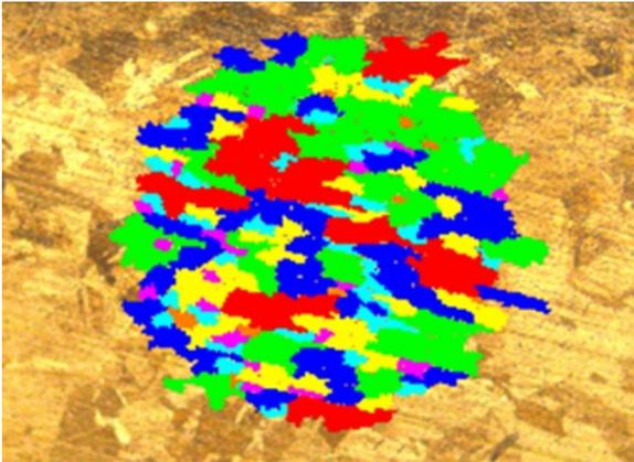
Fig. 2. Software grain measurement after mode №1 after stamping
