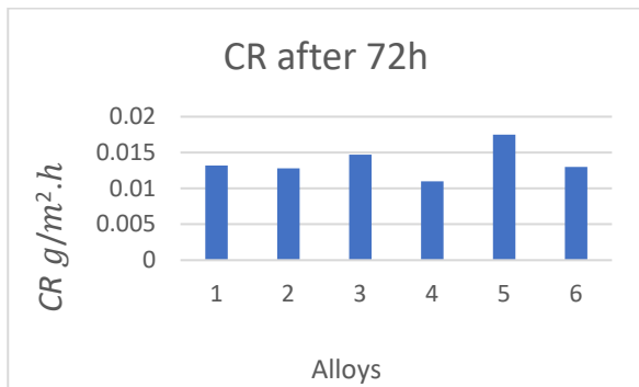
Fig. 3. Corrosion rate of AISi18Cu3CrMn alloy after 72h stay in H 2 SO 4
