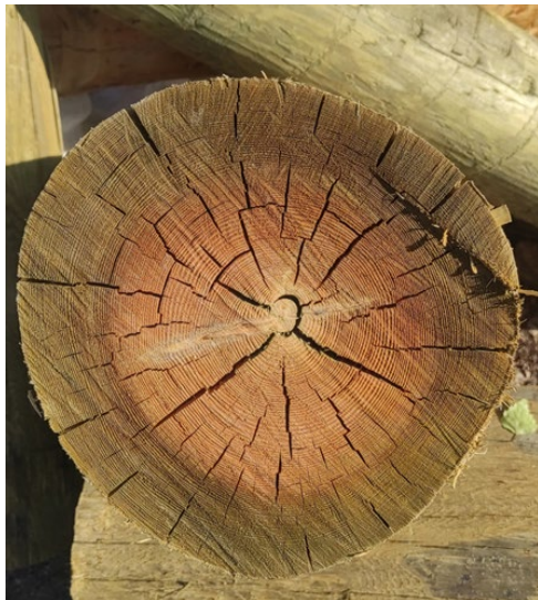
Fig. 1. Pinus sylvestris roundwood preservation with CCA when heartwood cannot be pressure impregnated
