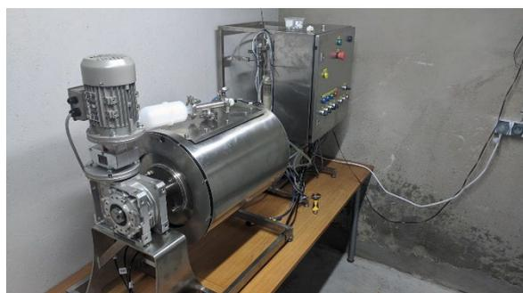
Fig. 3. SSF prototype reactor.
