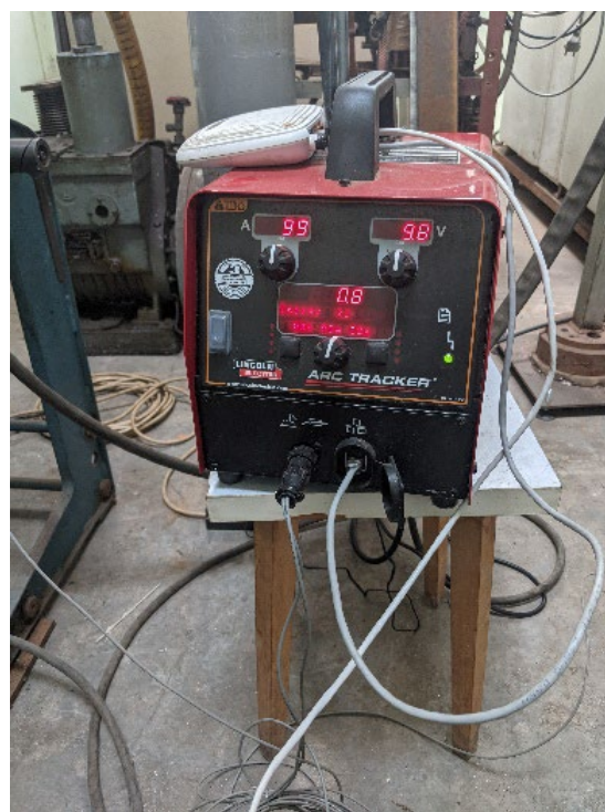
Fig. 6. Arc Tracker welding monitoring device.
