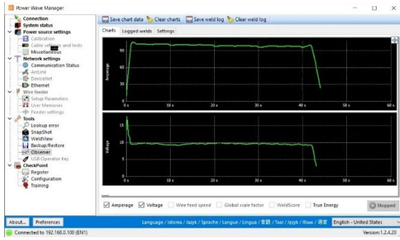
Fig. 8. Screenshot of captures current and voltage values with Arc Tracker welding monitoring device.
