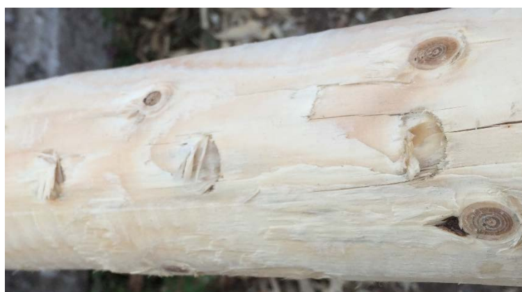
Fig.2. Roundwood surface damage caused by feed roller penetration in timber
