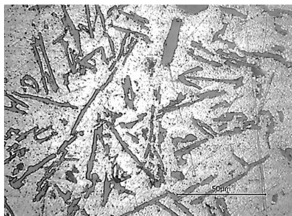
Fig. 6. Eutectic of phosphorus-modified AlSi18 alloy
