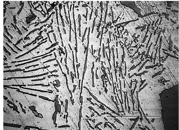
Fig. 1. Eutectic of unmodified AlSi18 alloy
