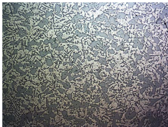
Fig. 2. Structure of modified by 0.04% P alloy AlSi25 x200
